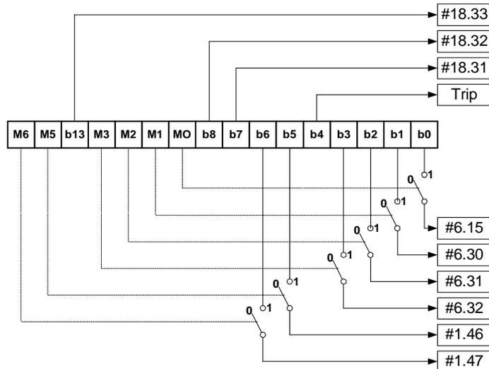
If mask bits M0 and M1 are set to 1, ENABLE and RUN FWD are updated with the values of b0 and b1 (either 0 or 1) every time the control word value is received. JOG and RUN REV will not be updated, even if the values of b2 and b3 change, because their mask bits (M2 and M3) are not set to 1. If M0 and M1 are reset to 0, the values in b0
