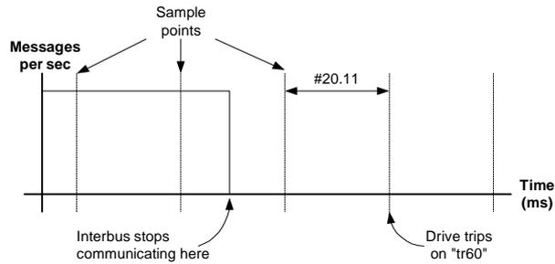
As can be seen from the diagram, the actual time from network loss to Drive trip will range from #20.11 ms to  $2 * \#20.11$  ms. By decreasing #20.11, the maximum trip time will be reduced, but if the trip time is set too low, spurious network loss trips will be seen.
