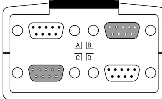
The pin connections for the Interbus Remote Bus IN and OUT connectors are given in the table below. 0V ISO is completely isolated from 0V COM.
