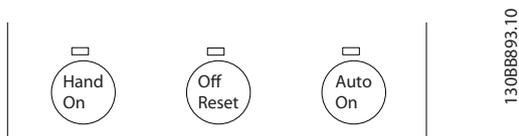
Local reference will force the configuration mode to open loop, independent on the setting of *1-00 Configuration Mode*.
