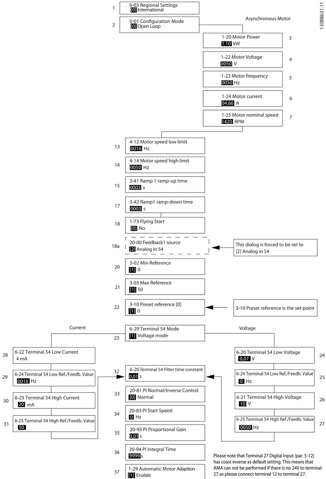
Please note that Terminal 27 Digital Input (par. 5-12) has coast inverse as default setting. This means that AMA can not be performed if there is no 24V to terminal 27 so please connect terminal 12 to terminal 27.
