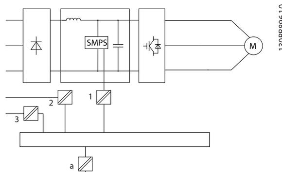
The functional galvanic isolation (a on drawing) is for the RS-485 standard bus interface.
