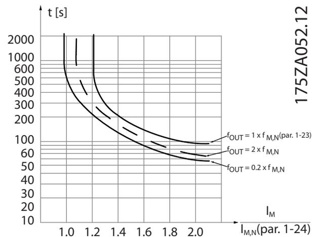
The X-axis is showing the ratio between  $I_{motor}$  and  $I_{motor}$  nominal. The Y-axis is showing the time in seconds before the ETR cuts off and trips the drive. The curves are showing the characteristic nominal speed at twice the nominal speed and at 0.2x the nominal speed.
