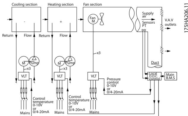
Illustration 2.6 Fan System Controlled by Frequency Converters
