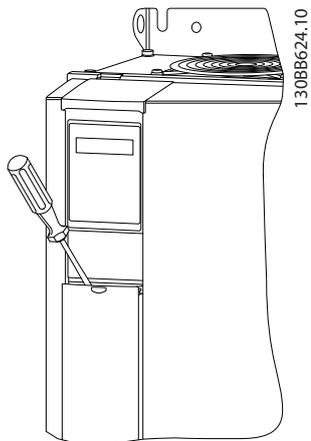
1. Place a screwdriver behind the terminal cover to activate snap.
