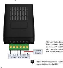
Alternatively (to External supply) the drives on-board 24V supply can be used (T1 (24V) and T7 (0V)) - Ensure total current consumption from T1 does not exceed 100mA.
